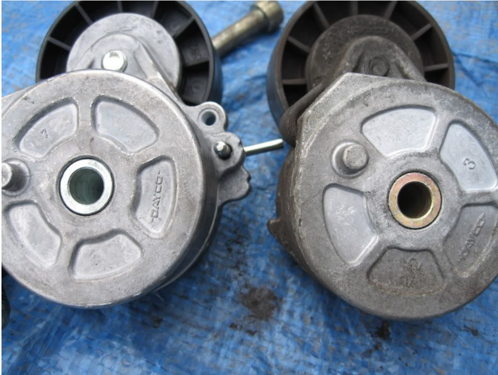
Old and new tensioners. Identical parts but new one not Pug supplied.
